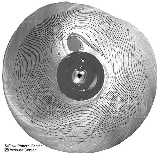
Fig. 1 Flow pattern on the back casing wall opposite the impeller, overlaid with isobars
